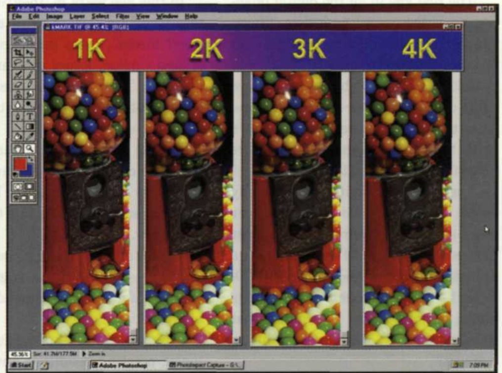
Zoom-in of individual images scanned at 1000, 2000, 3000 and 4000 line resolution
